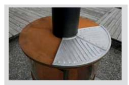
The combustion chamber in the SURPRISE is made from high-quality Corten steel. Set up unprotected outdoors, the Corten steel, delivered blank, develops surface rust within a few months and forms a strong protective layer underneath, which protects the steel against fast deterioration. The intensive orange-brown colour looks great and creates an aesthetically exciting contrast with the black varnished base and flue as well as the solid cast iron grill plates.
